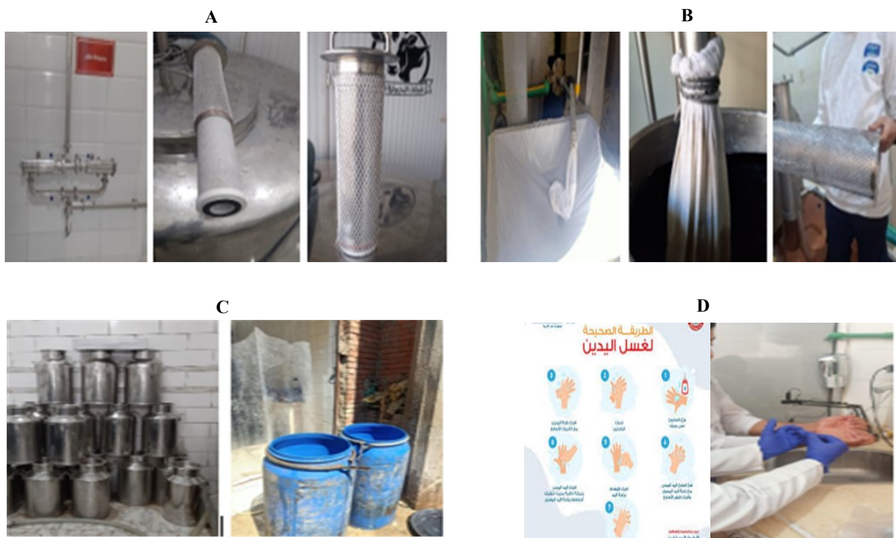
Figure (2). Implementation of Technical and Hygienic Interventions in the Milk collecting center (A–B) Upgrade of the milk filtration system (traditional filter vs. stainless steel fine-mesh system). (C) Replacement of plastic containers with stainless steel (AISI 304). (D) Implementation of GMP training in accordance with ISO 22000:2018 requirements.
