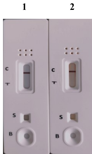
Fig. (7). Specificity of LFIA assay using direct culture of rough Brucella strains: (1) Brucella abortus biovar 1 (vaccine strain RB51), (2) B. ovis REO198 both were in a colony count of 1-5 \times 10^8 CFU/ sample.
